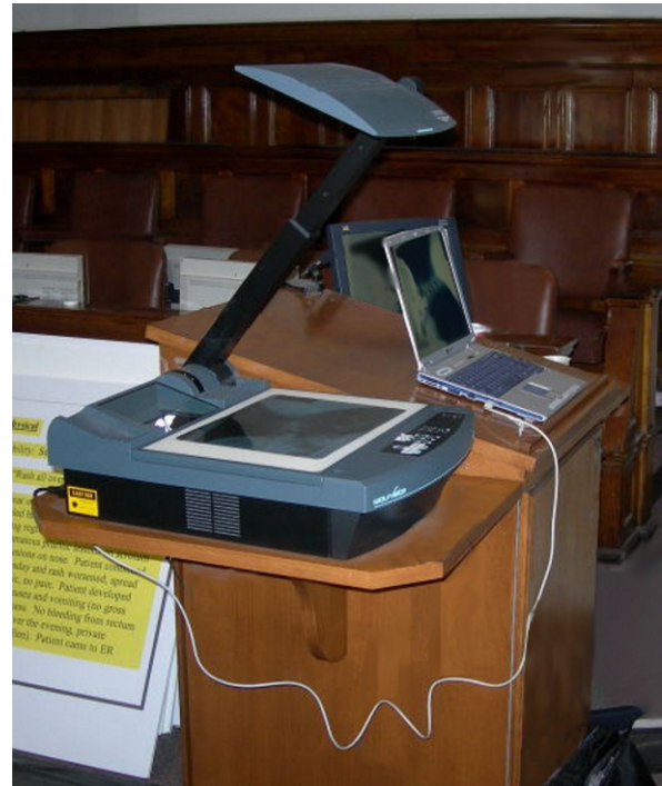
The Professional Visualizer picks up images with 3-CCD's true color and contrast, that can play a deciding role in malpractice suits at the NYS Supreme Court. Here, the Visualizer is connected to a laptop and picks up an image from an x-ray that is displayed on the screens of the judge, jury and lawyers. No more time consuming need to pass around evidence.
