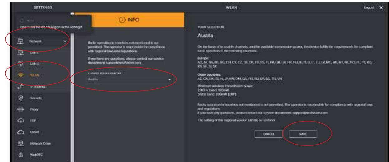
In the Cynap settings menu under "Network" -> "WLAN" the region, in which the Cynap is operated, must be selected.
