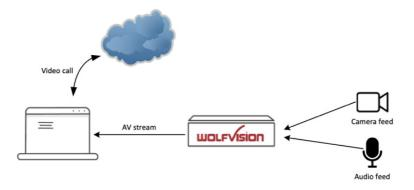
Laptop/PC (only) uses OS installed MS Teams and Zoom app and uses Cynap attached AV resources via vSolution App.
