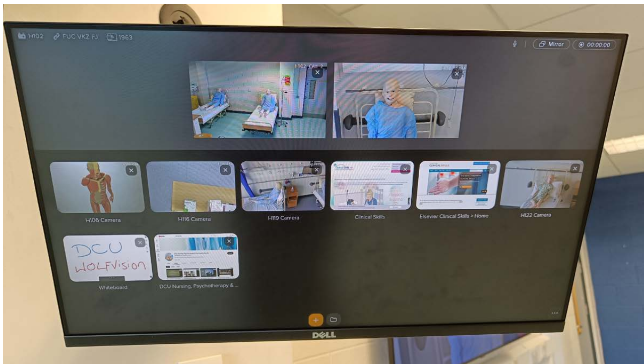
vSolution COMPOSER for Cynap Pro enables simple control of content on dual display screens. Multiple content sources can be prepared in the lower part of the screen and then drag-and-dropped onto either left or right display screens when required during classroom sessions.
