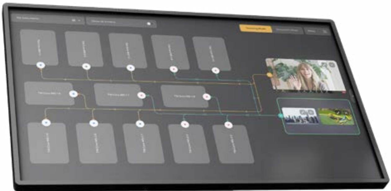
Sample Room View configured for twin main display screens, with content easily identified using different colours and either one or two arrows for each stream.
