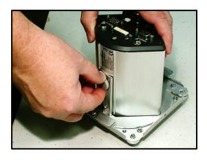
8) Install camera into the assembly using ¼ - 20 knurled screws (supplied with camera).
