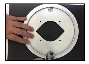
18) Attach alignment ring to face-plate with Nuts (G) provided.
