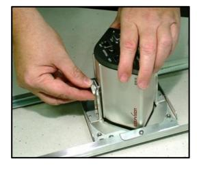
9) Install camera into the assembly – tighten ¼ - 20 knurled screws (supplied with camera).
