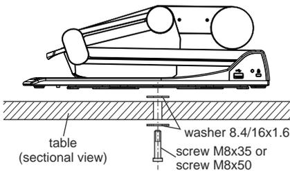
The Visualizer can also be fixed onto a table with the supplied table lock bolt in order to minimize the risk of theft.
