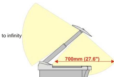
In this way it is also possible to make recordings of subjects in the room or surrounding area, as with a video camera by just tilting the top mirror.
