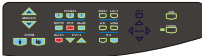
Control panel in "unit on" position, text enhancement and macro function activated - camera menu and help not visible
