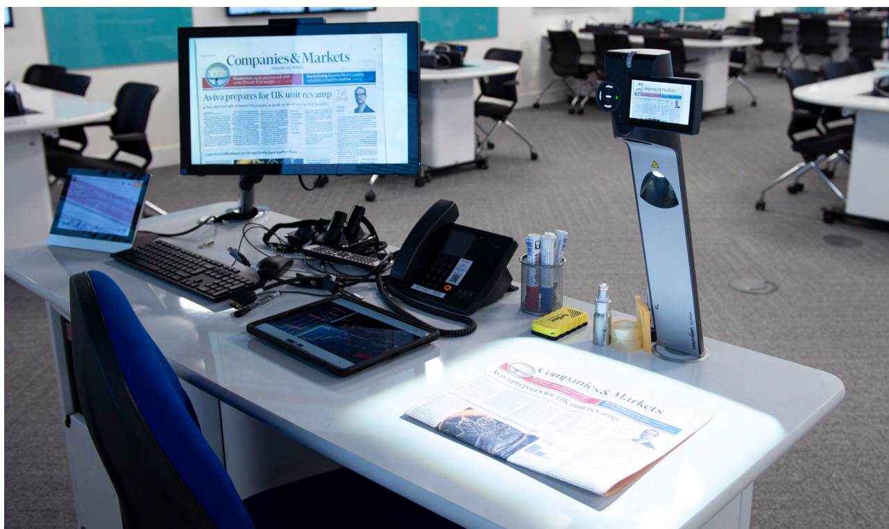
Handwritten notes and physical content of all kinds can be displayed on screens throughout the room using the WolfVision VZ-8Neo+ Visualizer.
