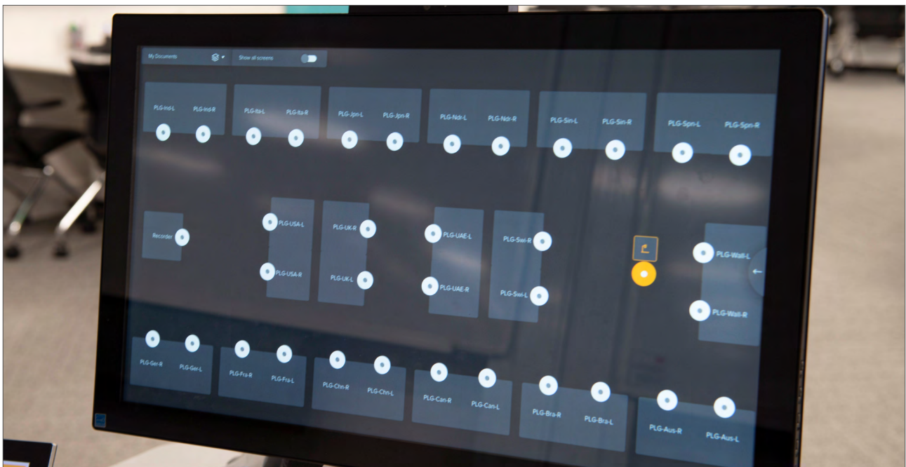
The 'Room View' is customisable to match exactly the workstation layout. Files can be sent to workstations, and simple drag and drop functionality enables content to be easily pushed and pulled between screens as required.
