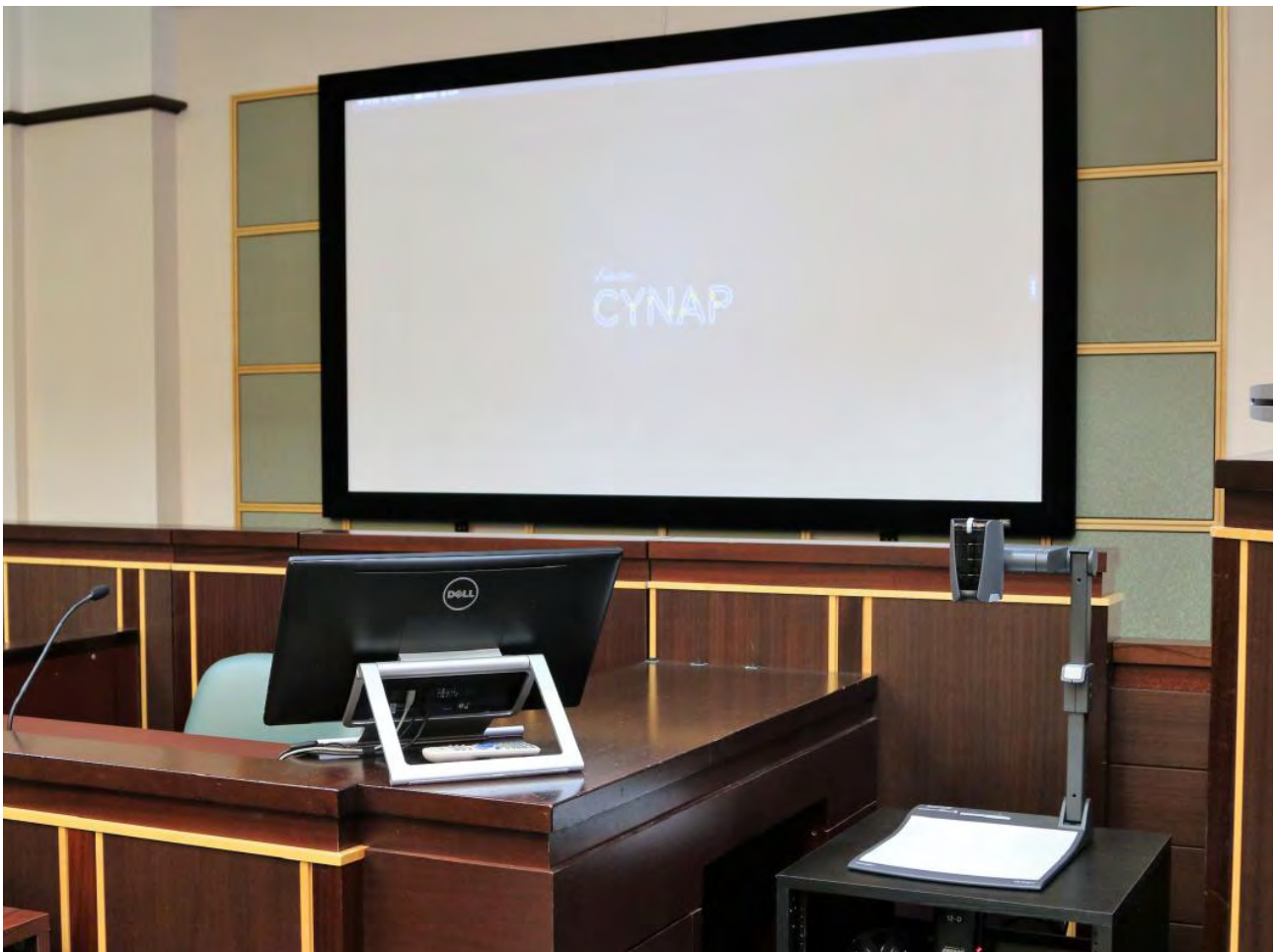
With 2x HDMI Out ports, content can be displayed both on the main display screen and previewed on the judge's monitor.
